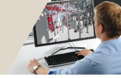
Modeling the Hilti MEP Supports as designed in the Hilti Design Core and/or the Hilti Design Specifics. The Hilti delivered model is passed through an engineering quality control and respectful of the Project BIM models. Any applications uncovered to be beyond the scope of the Design Core or for which Hilti has not provided a design will be marked accordingly in the BIM model, but will not be modeled.
