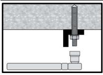
Loading the anchor after required curing time tcure the anchor can be loaded. The applied installation torque shall not exceed T<sub>max</sub>.
