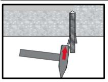
Setting element for overhead applications, observe working time "twork"
